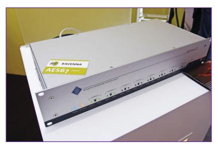
The Neumann DMI-8, an eight-channel AES42 digital microphone interface, will be available with a dual-port RAVENNA interface option. This is effectively the first completely networked audio signal chain from the acoustic sound source.
