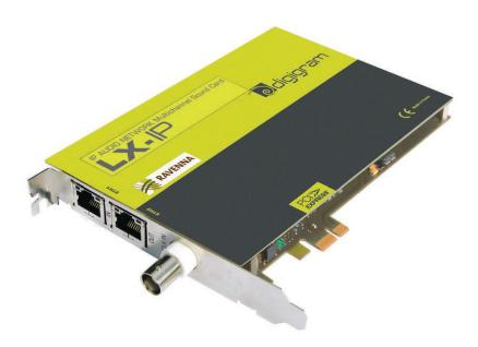
French company Digigram introduced the LX-IP RAVENNA PCIe sound card, its first RAVENNA/AES67-enabled product, supporting a latency down to one audio sample per IP packet and up to 256 RAVENNA I/O channels from multiple RAVENNA streams. It is ideal for high-density audio production or automation applications in radio and TV broadcast studios.
